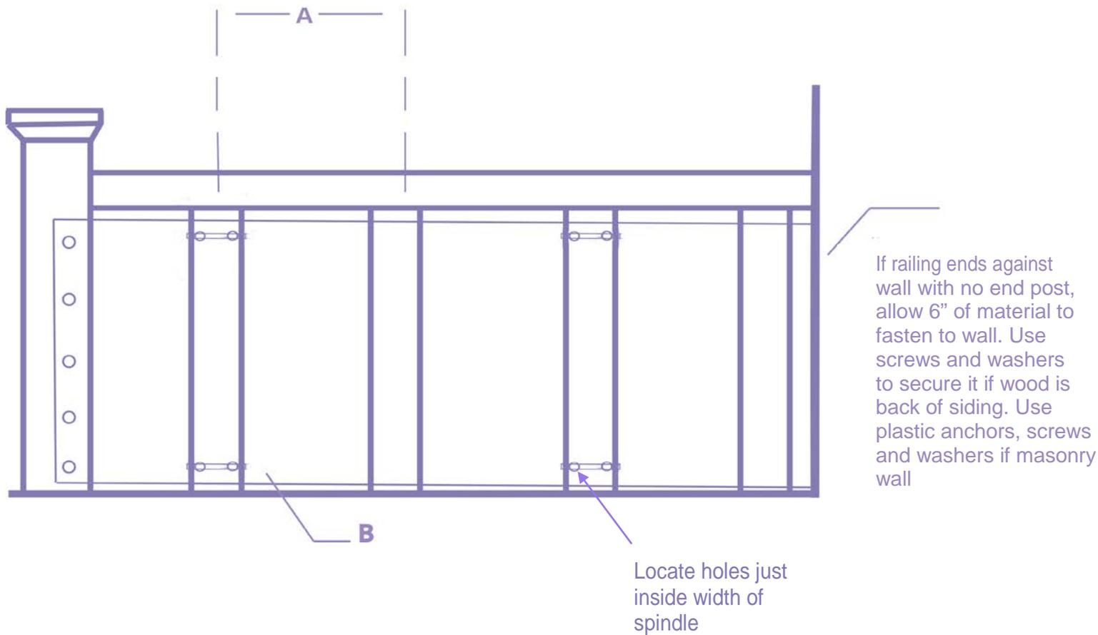
**A. While it is not necessary to fasten Outdoor Rail Guard to every spindle, do not leave more than 12" between attachments.**
